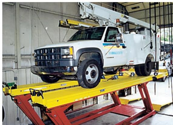
Any type of vehicles can be lifted from utility vehicles to buses to emergency vehicles. All OMER parallelogram lifts models are available in either continuous base or open floor design and can be installed either surface, flush or flush in a recess.
