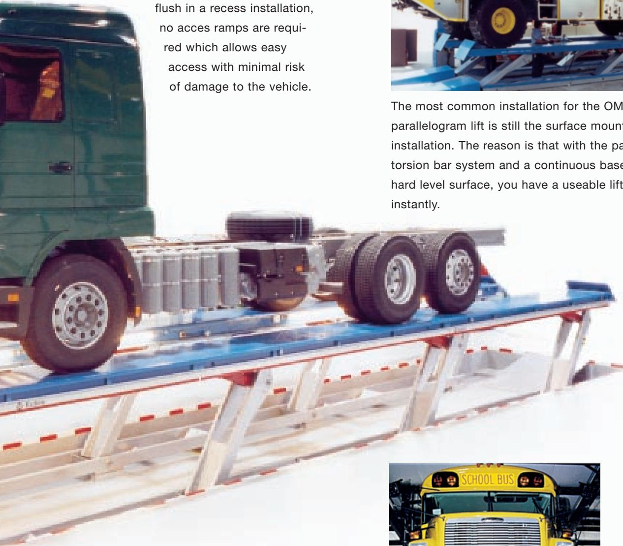
The OMER parallelogram can lift various vehicles with weights ranging from 26,400 lbs to 115,000 lbs. OMER's versatility also allows wheelbases varying from 23 to over 42 feet.
