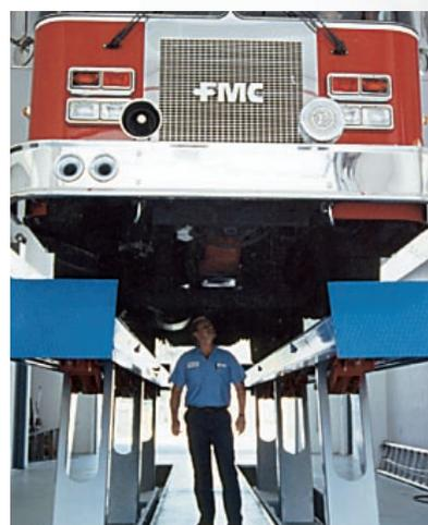
The OMER parallelogram lifts offer the highest overall lifting height of just about any heavy-duty lift available worldwide. The 73-inch height is a full 10 inches higher than the 63 inch lifting height of OMER's only competitor in the parallelogram market. That extra 10 inches will make the OMER parallelogram lift the clear choice.
