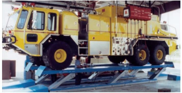
The most common installation for the OMER parallelogram lift is still the surface mounted installation. The reason is that with the patented torsion bar system and a continuous base on a hard level surface, you have a useable lift instantly.
