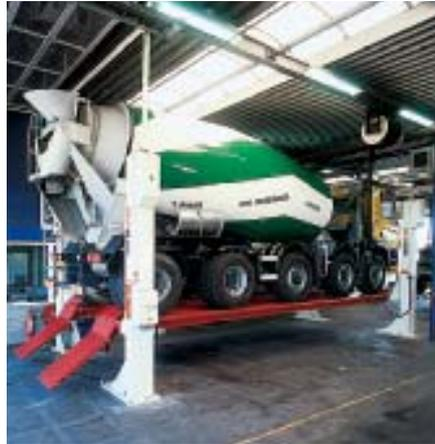
The ST4250 can be used for lifting all types of heavy vehicles as well as multi-axle vehicles.
