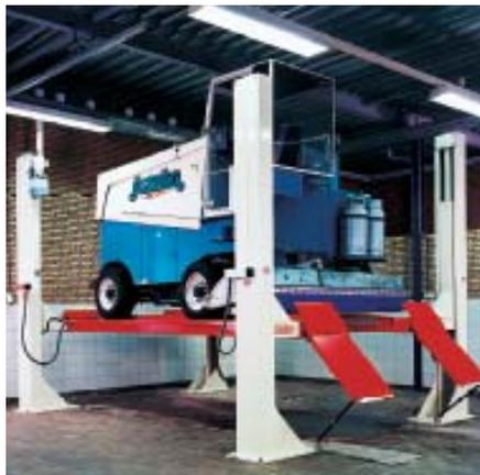
With the platforms being available in several lengths, vehicles with different wheelbases can be lifted.
