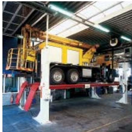
For lifting articulated buses, trucks with semi-trailers and articulated units, connected versions are available. The two vehicle lifts set up in-line can be used both synchronously or separately.
